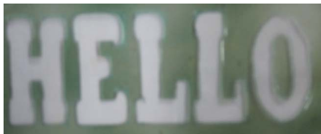
Figure 9 Appearance of cured film of APSUA system with image. Composition of the system: APSUA : DPGDA : 1173 = 60 : 40 : 0.0007(wt.). [Color figure can be viewed in the online issue, which is available at wileyonlinelibrary.com .]
